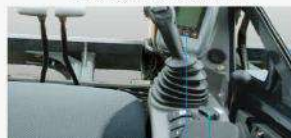
Shown equipped with auxiliary function lever and cab as optional items. ECO / PWR mode selector switch Engine control dial
